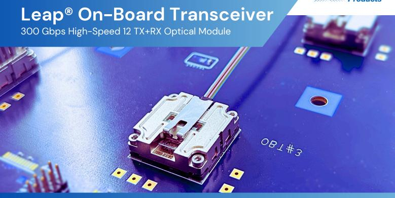
Amphenol AOP 300 Gbps Leap® OBT High-Speed 12 TX+RX Optical Module is faster, smaller, more cost and power efficient than most conventional datacenter interconnects. With its 12 channels independently and each channel delivering up to 25 Gbps, it is versatile, aggregating up to 300 Gbps. It is the best choice for high density projects that need to take advantage of board space while being as close as possible to the FPGA.
