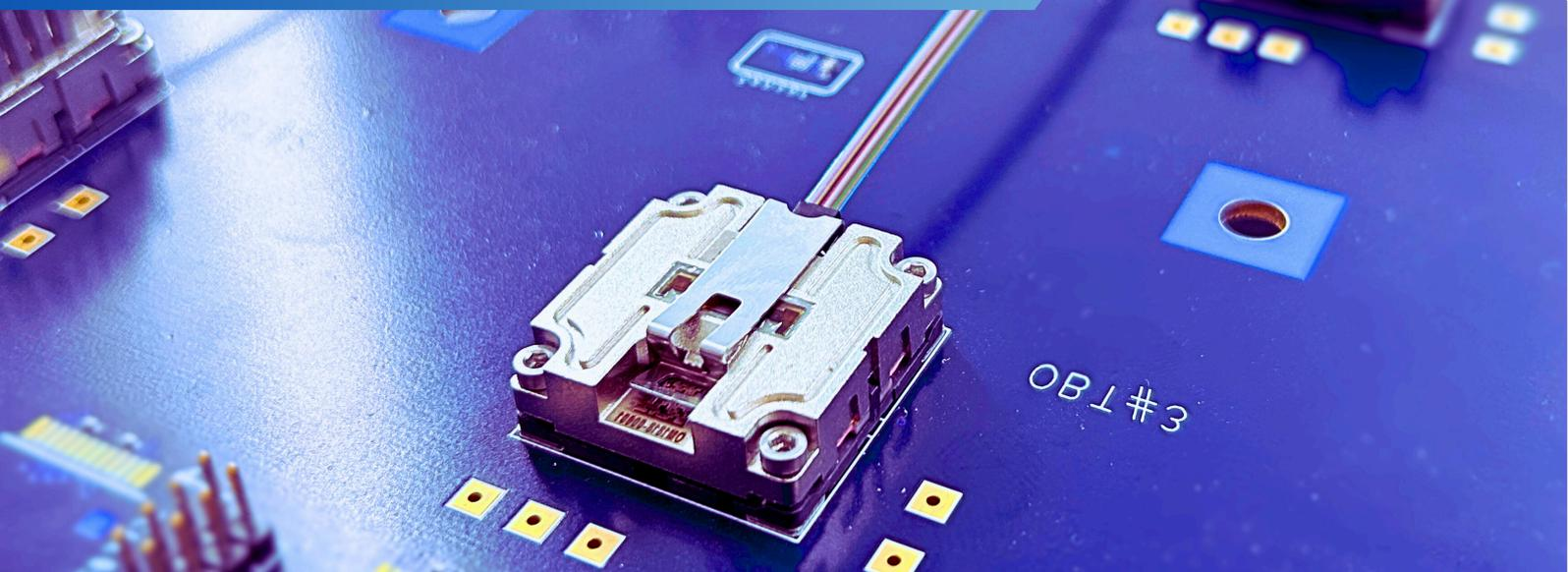
Amphenol AOP 300 Gbps Leap<sup>®</sup> OBT High-Speed 12 TX+RX Optical Module is **faster, smaller, more cost and power efficient than most conventional datacenter interconnects**. With its 12 channels working independently and each channel delivering up to 25 Gbps, it is versatile, aggregating up to 300 Gbps. It is the best choice for high density projects that need to take advantage of board space while being as close as possible to the FPGA.
